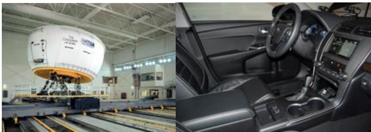
Figure 4. Exterior and interior views of the NADS-1 simulator.
